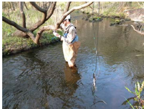
The Hester-Dendy sampler is in the water, being tied off to a tree as the multi-parameter probe takes readings at Hogtown Creek upstream of the Haile Sink location.
